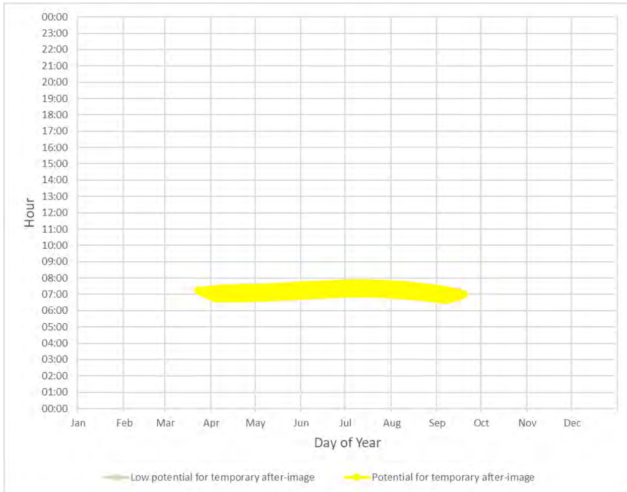
Figure 6: Time of Glare Hazard for Observation Point 10 – Bike Path
