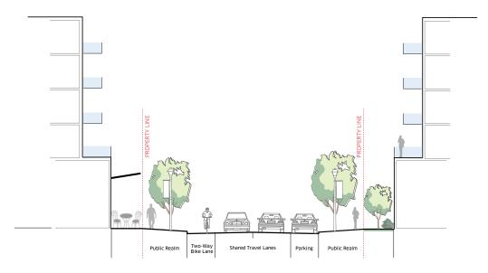
Figure 15 Conceptual Pedestrian Oriented Street - Parking on One Side with Bike Lane (20 m)
