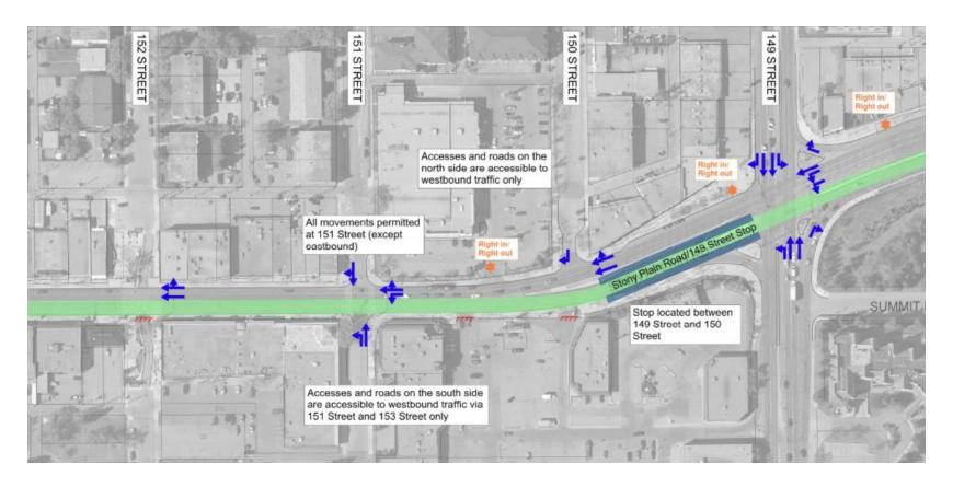
Option 4 - One-Way Roadway, LRT South Alignment with 1 Westbound Through Lane and Wider Sidewalks This option's design includes south side running LRT alignment with one westbound lane and approximately 3 metre wide sidewalks and amenity spaces.
