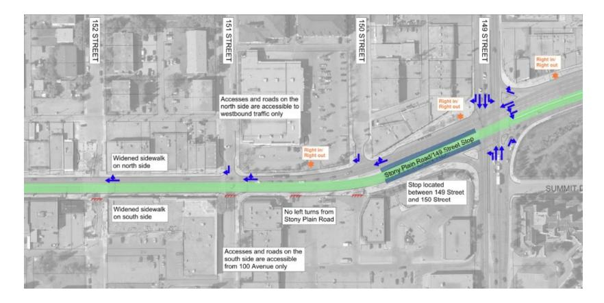
Option 5 - Two-Way Roadway, LRT Centre Alignment with 1 Lane Each Direction
