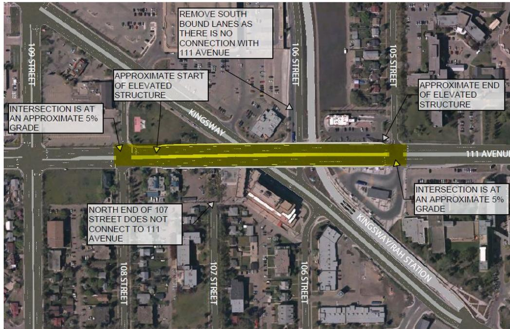
**OPTION A.2 – Grade Separation (showing 111 Avenue At-Grade with LRT Elevated)**
