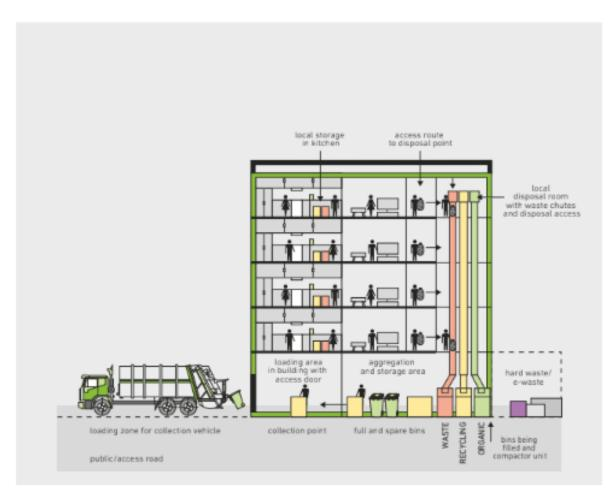
Diagram showing three chute systems in multi-unit building (source: <u>Waste and recycling in multi-unit developments</u>, Victoria State, Australia).
