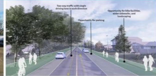
Future one-way driving lane in each direction with parking on each side of the road. Opportunity for bike facility, wider sidewalk and landscaping.
