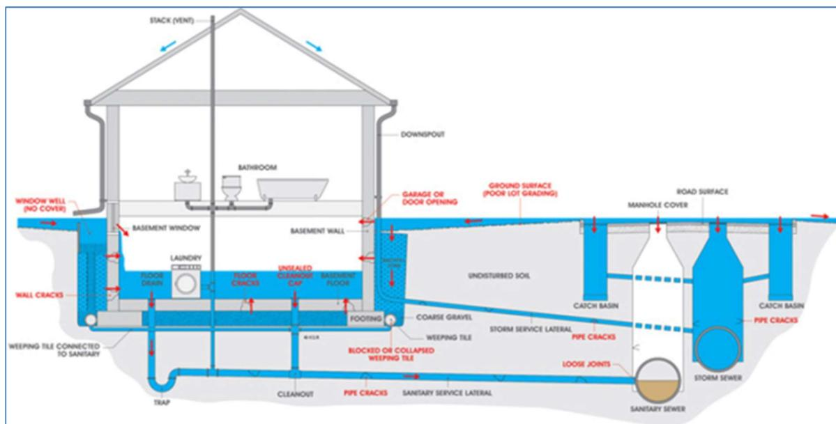
The longer the duration that the water pools on the ground surface after a storm event the higher the risk that the water will access the sanitary pipes and/or foundation drains of properties without adequate flood proofing and enter the building. The SIRP Secure theme was developed to address each of these pathways through three focus areas for intervention:
