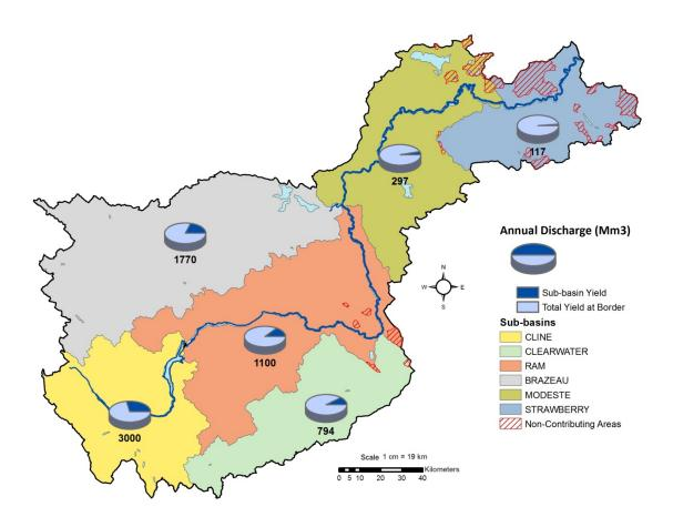
Figure 6. Water Yield Data for Sub-basins in the NSR watershed (modified from Golder 2008). Pie charts show the fraction of total water yield at the AB-SK border attributable to the sub-basin. The figure shows that the majority of the water yield is from upstream in the watershed.
