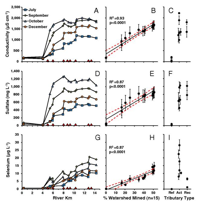
Figure 7. Showing watershed areas mined and concentrations of selenium, sulfate, and conductivity from Lindberg et al. 2011.
