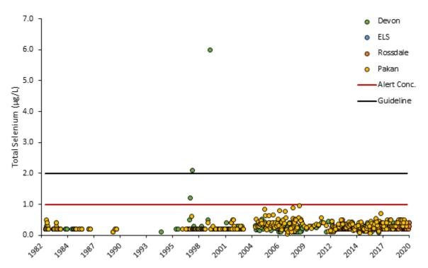
Figure 8. Selenium concentration (µg/L) in the NSR at Devon LTRN Site, Pakan LTRN site, and EPCOR's Water Treatment Plant intakes from 1980 to 2020.
