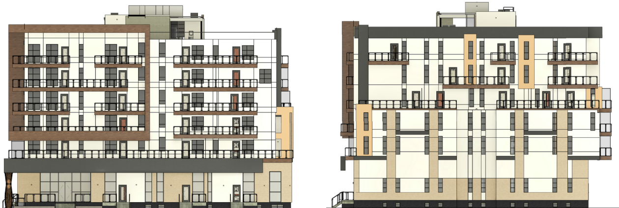
SOUTH (RIGHT) AND EAST (LEFT) ELEVATIONS OF THE DC2 PROVISION SHOWING THE RESTRICTIONS ON BALCONIES AND OPENINGS ON THE LOWER 13 METRES OF THE EAST FACADE FACING THE NEIGHBOURING BUILDING
