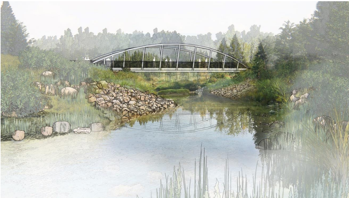
Plate 4.3. Conceptual Plan View of Proposed Steel Tied-Arch Bridge Design at Smith Crossing (Provided by: Morrison Hershfield, City of Edmonton and EDA Planning + Urban Design 2021)
