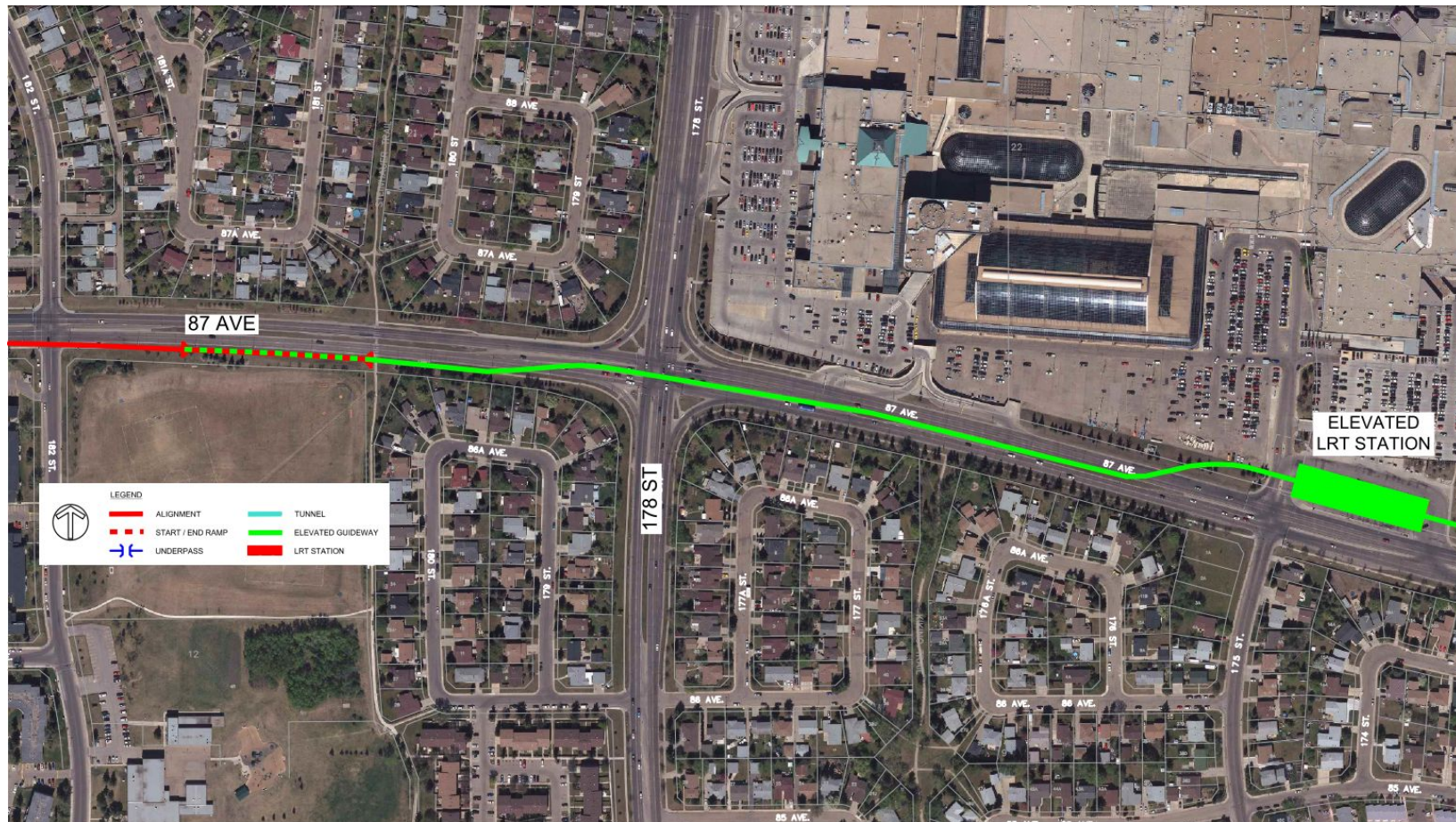
Elevated LRT Guideway, Median Alignment
