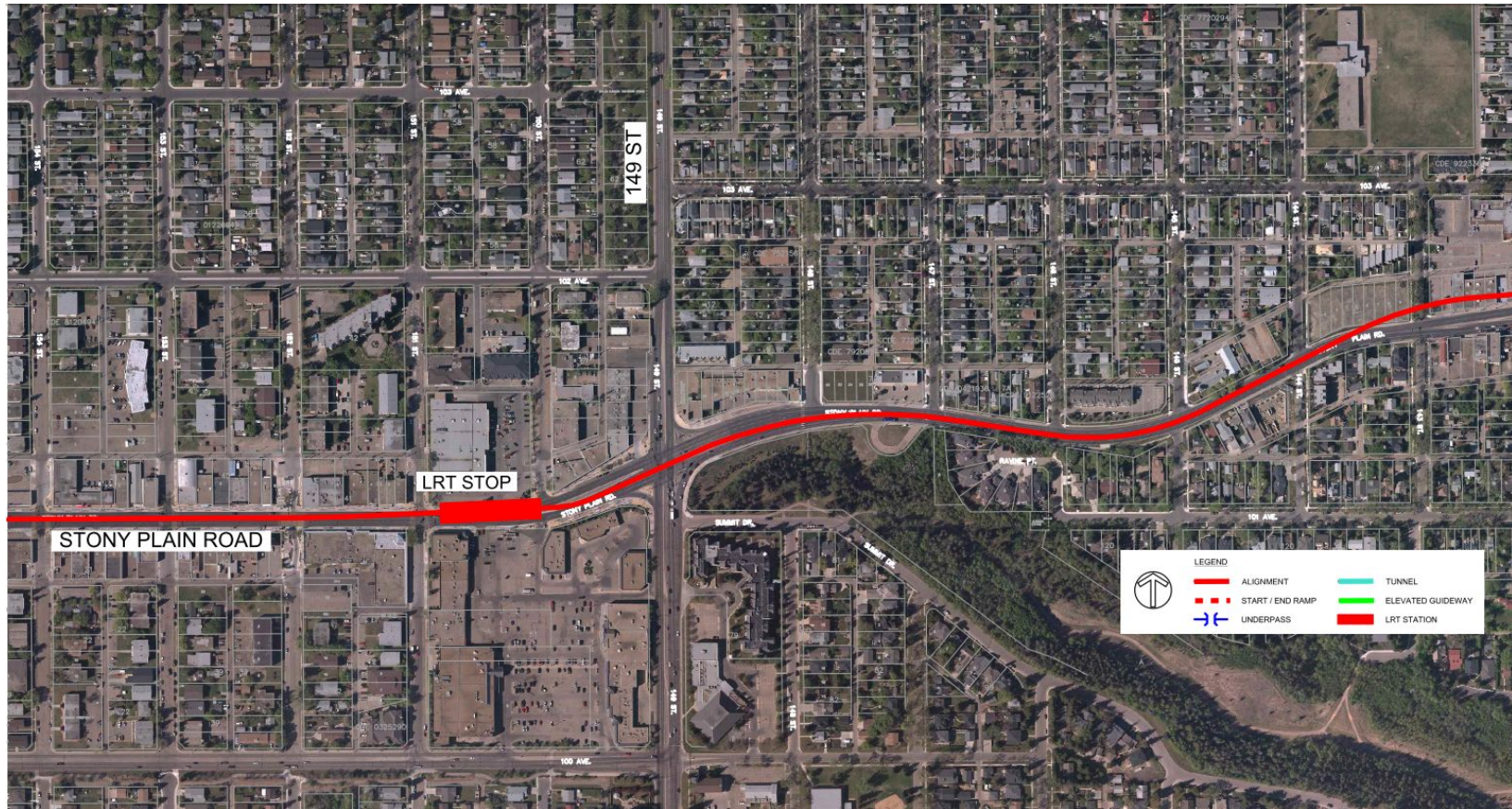
At-Grade LRT, Center Alignment
