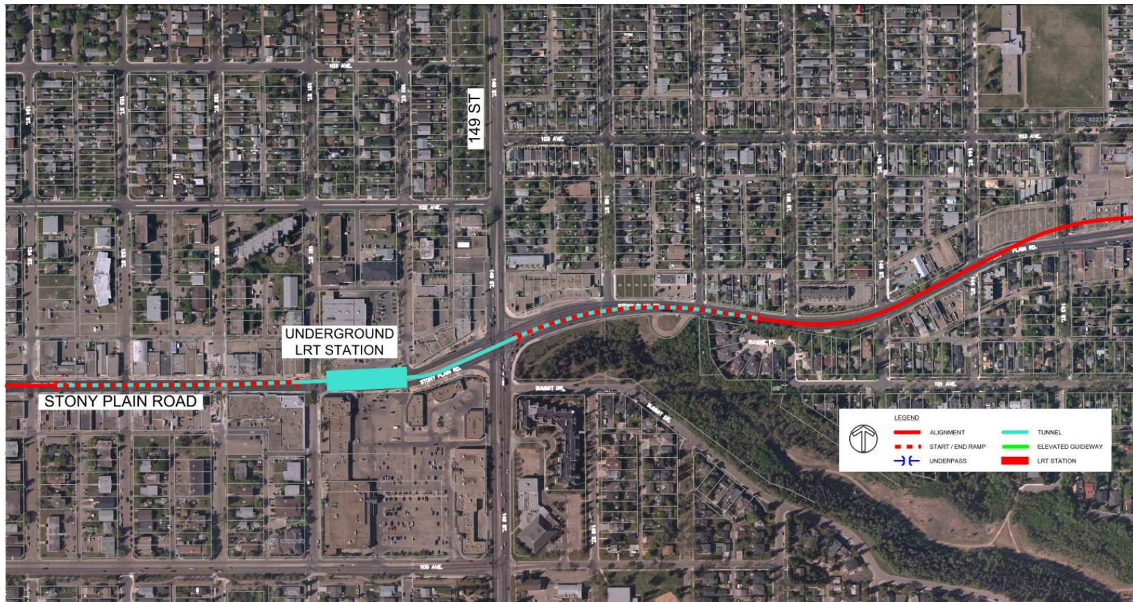
Underground LRT, Center Alignment
