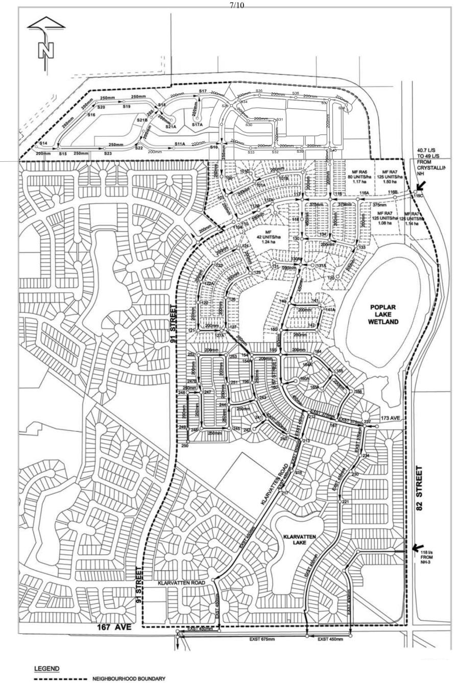
EXISTING SANITARY SEWER PROPOSED SANITARY SEWER
