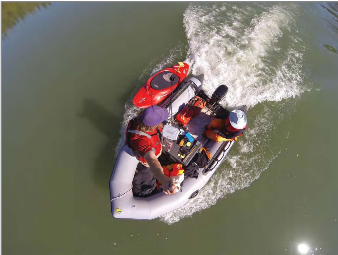
Photo 1: Bird's Eye View of Bathymetry Survey Vessel. Note kayak with GPS unit mounted on top. The GPR and sonar heads were mounted inside the kayak, while all topside electronics were contained in the zodiac.
