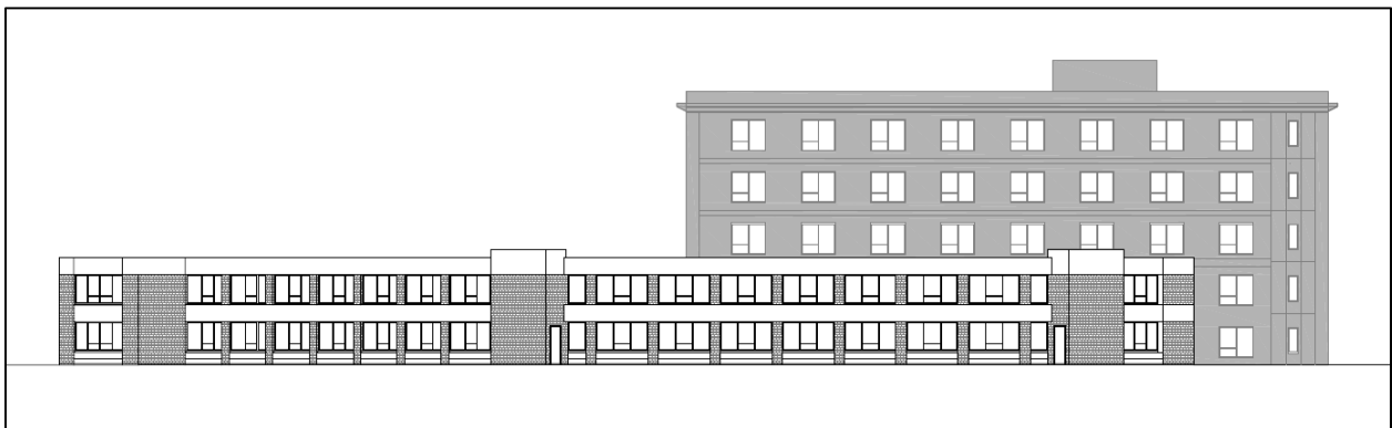
NORTH ELEVATION: EXISTING TWO-STOREY DEVELOPMENT AND PROPOSED FIVE-STOREY EXPANSION
