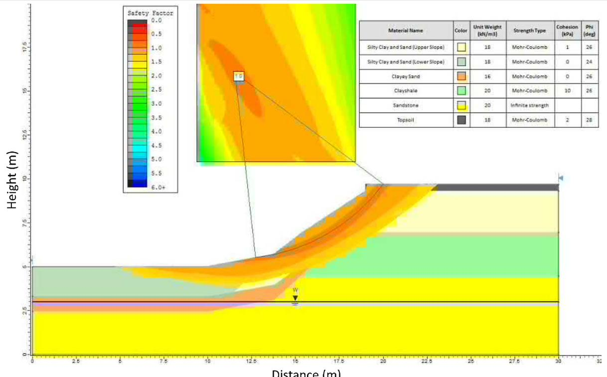
Failures with factor of safety of 1.5 or less shown
