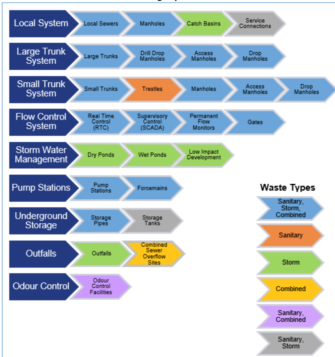
Figure 3.1.1-1 EWSI's Drainage System Overview
