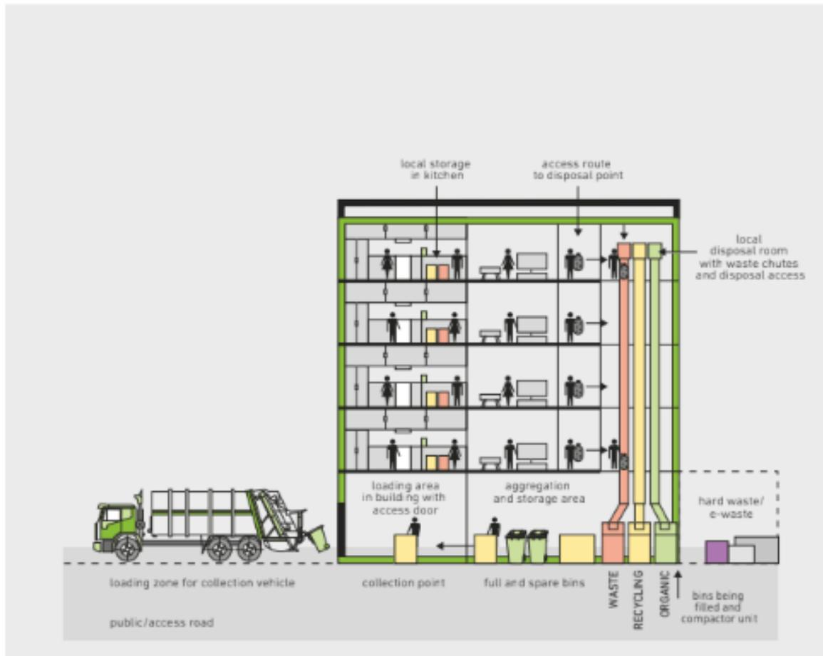
Diagram showing three chute systems in multi-unit building (source: [Waste and recycling in multi-unit developments](#), Victoria State, Australia).
