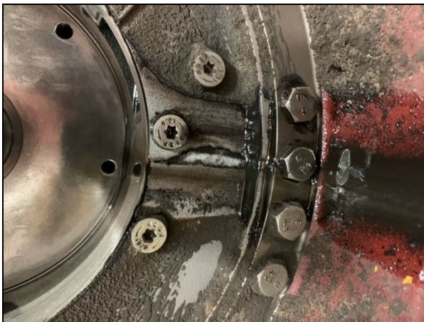
Figure 3: Metal contamination inside the transmission.
