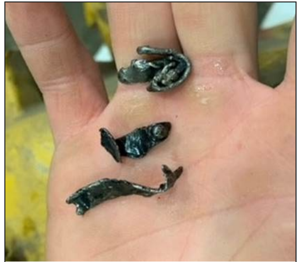
Figure 2: Metal debris from inside the torque converter housing.
