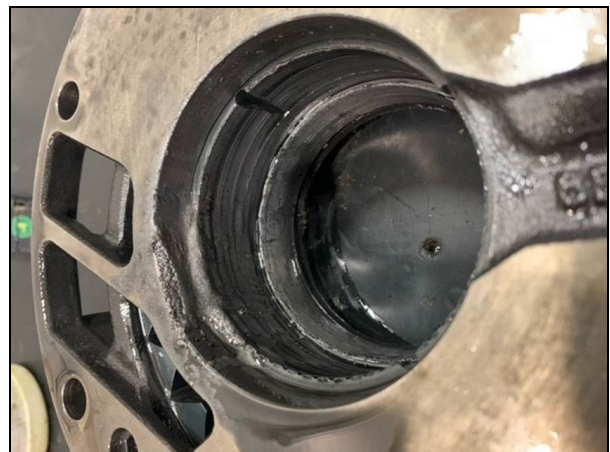
Figure 4: Damage inside the transmission oil pump.
