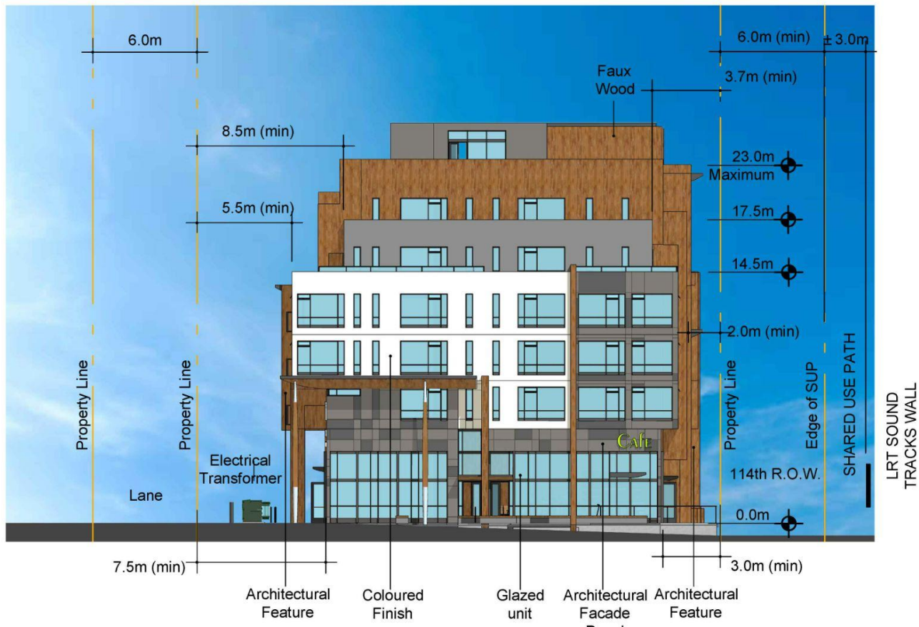
APPENDIX 7d (North Building) - SOUTH ELEVATION
