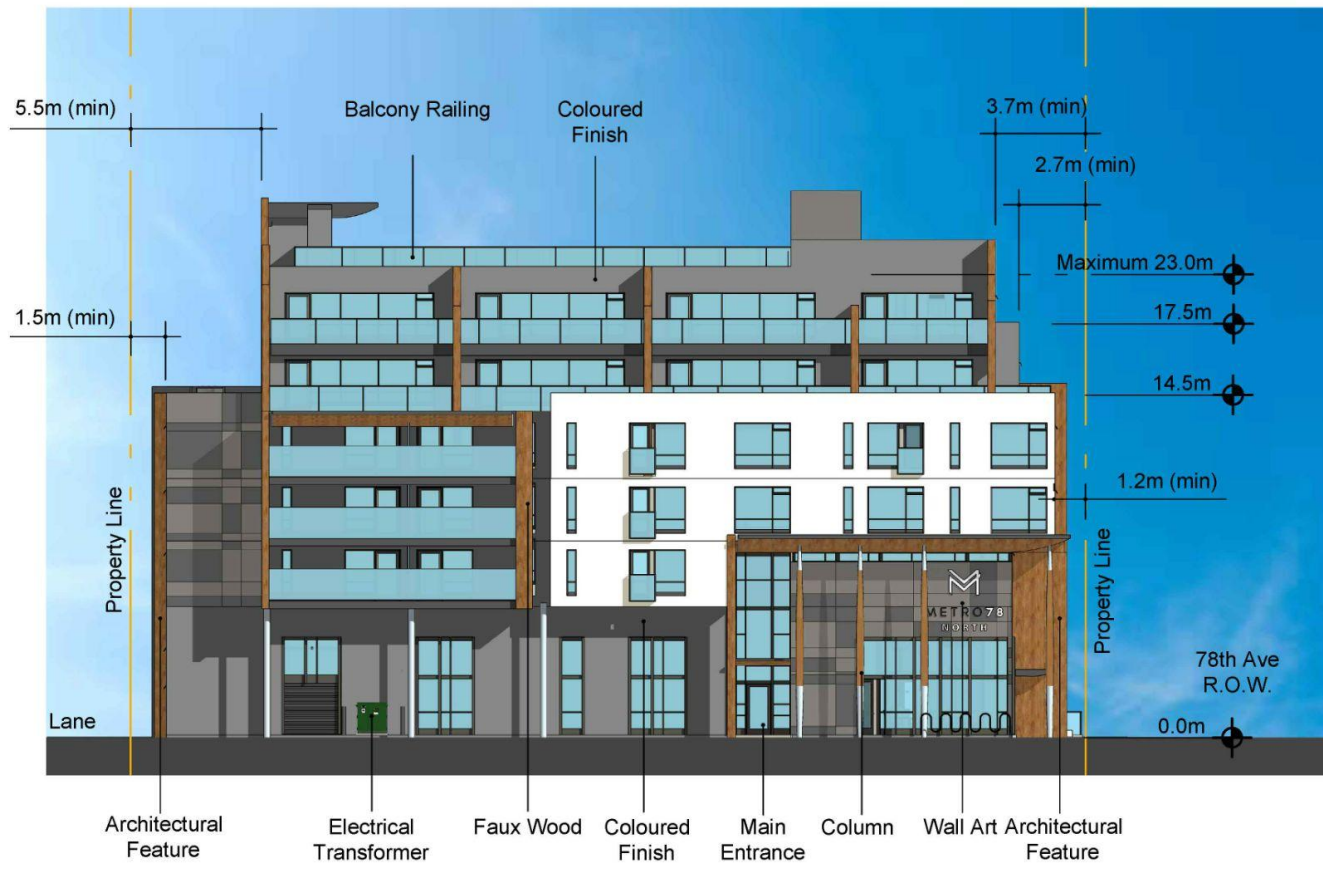
APPENDIX 7b (North Building) - WEST ELEVATION
