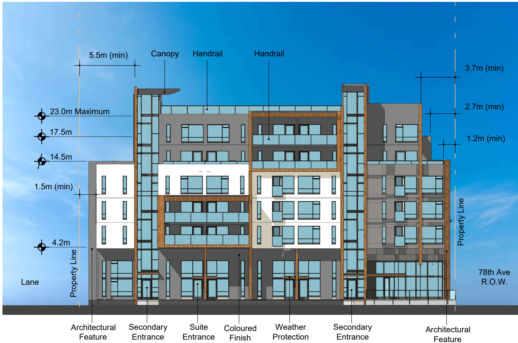
APPENDIX 8a (South Building) - EAST ELEVATION
