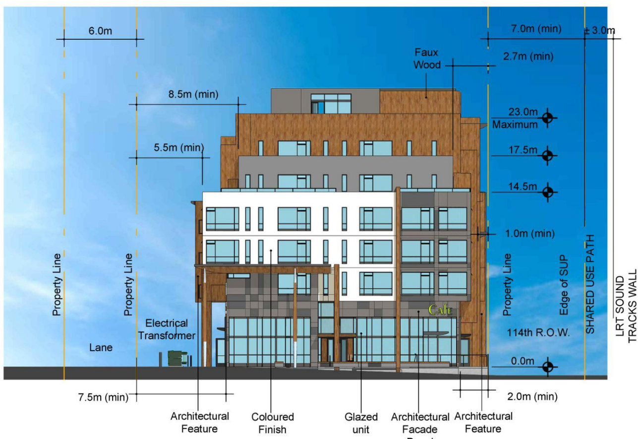
APPENDIX 7d (North Building) - SOUTH ELEVATION
