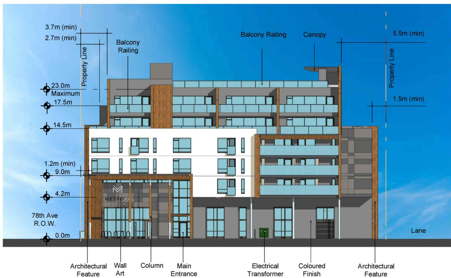
APPENDIX 8b (South Building) - WEST ELEVATION
