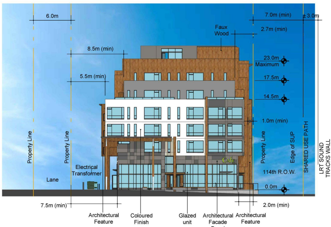
APPENDIX 7d (North Building) - SOUTH ELEVATION
