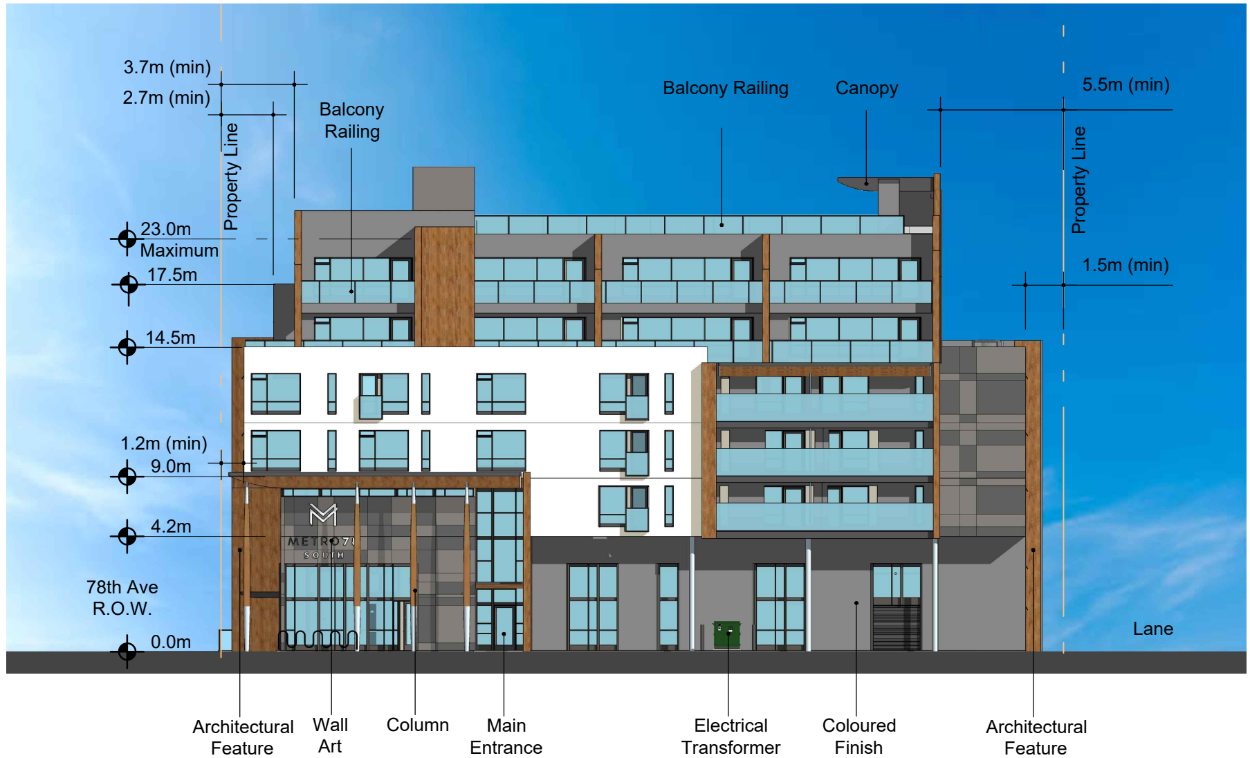
APPENDIX 8b (South Building) - WEST ELEVATION
