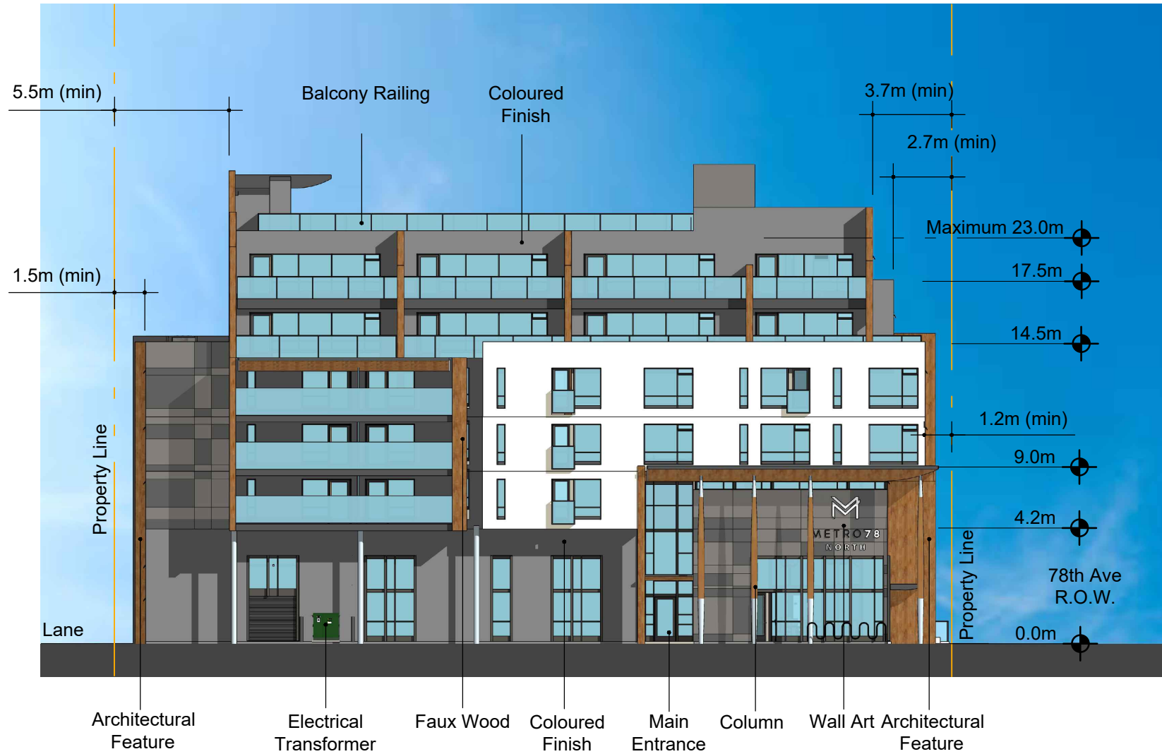
APPENDIX 7b (North Building) - WEST ELEVATION
