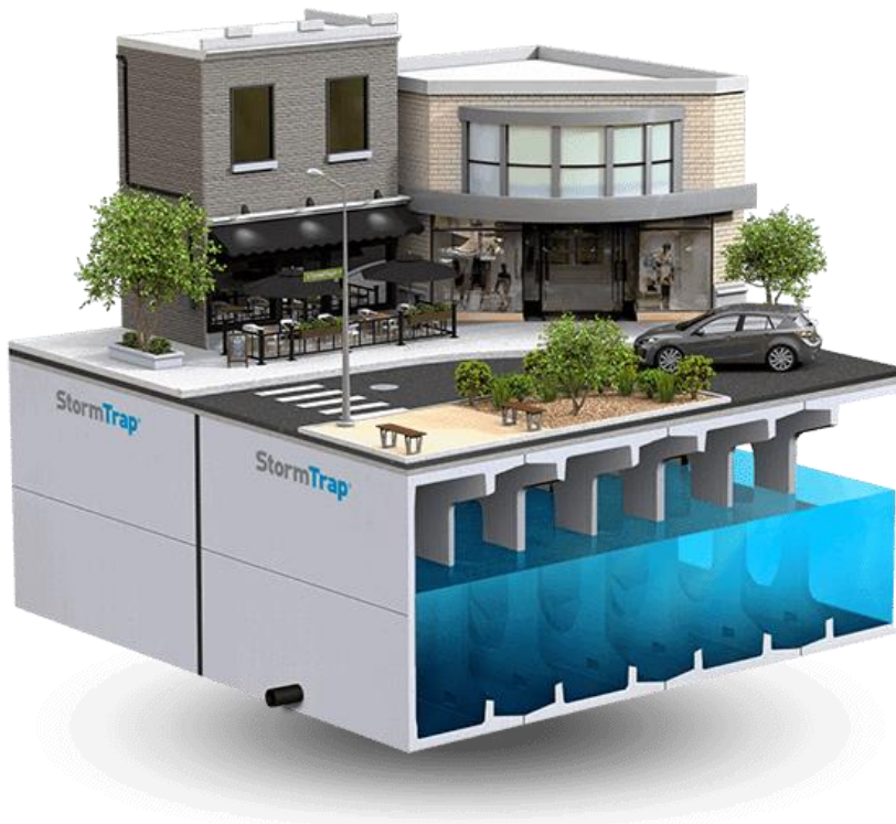
Figure 2. Underground Storage System Schematic. Modified from: Stormtrap, 2022.
