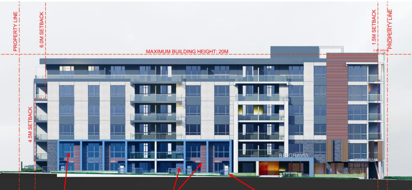
Extending panels and frames to the second level makes the unit look like two storeys from the outside.
