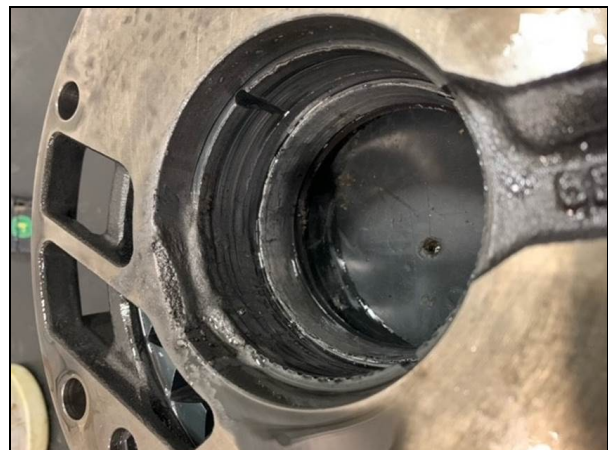
Figure 4: Damage inside the transmission oil pump.
