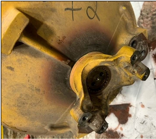
Figure 1: The torque converter input bearing showing the heat-affected area.
