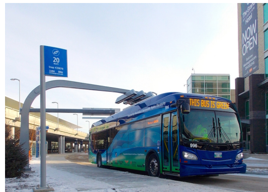
Figure 7.2 Winnipeg's en-route charging equipment with a New Flyer bus
