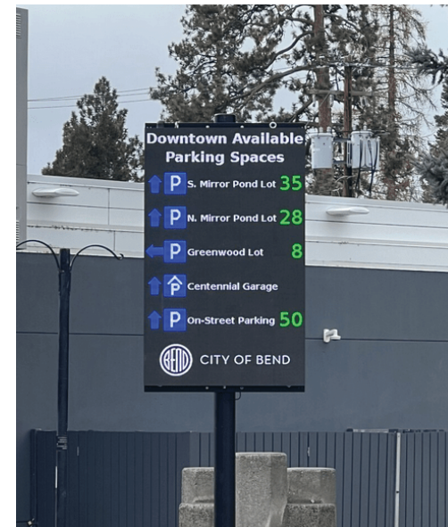
IMAGE DIGITAL WAYFINDING SIGNS INSTALLED IN BEND OREGON HELP PREVENT PEOPLE CIRCLING TO FIND AVAILABLE PARKING.
