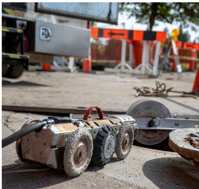
Televising equipment for inspecting wastewater pipes
