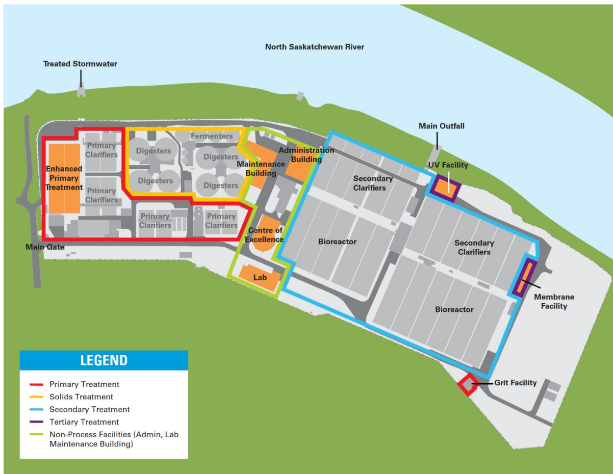
Figure 3.2.1-1 Gold Bar Wastewater Treatment Plant Overview
