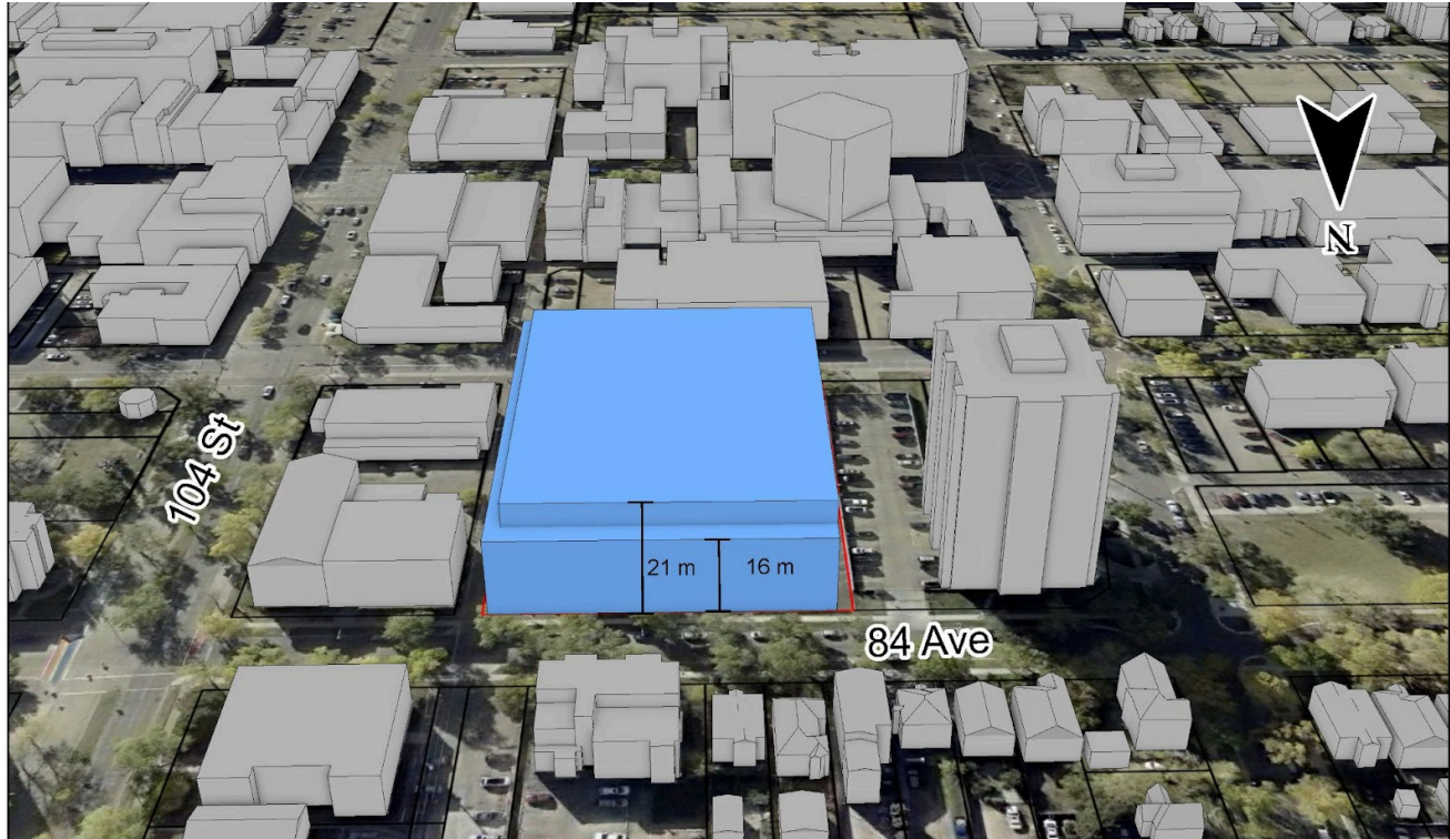
3D Model of proposed MU h30.0 f5.5 Zone showing maximum floor area ratio, minimum setbacks and reduced height
