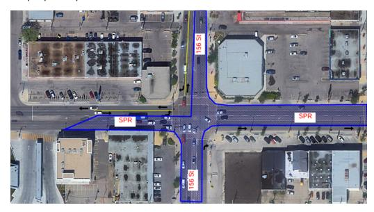
This partial closure will not accommodate any north/south and east/west through traffic with limited turn movement capacity remaining. The eastbound to northbound and northbound to eastbound left turns will be maintained.
