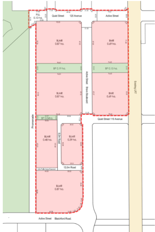
Conceptual plan showing the proposed roads, street classifications, greenway connections (green), and the Metro LRT corridor (yellow).
