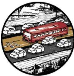
Dedicated Right-of-Way Bus-only lanes fully segregated from mixed traffic
