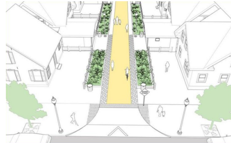
Example of a Shared Alley – NACTO Manual National Association of City Transportation Officials (NACTO)
