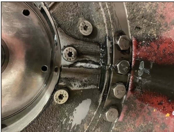
Figure 3: Metal contamination inside the transmission.
