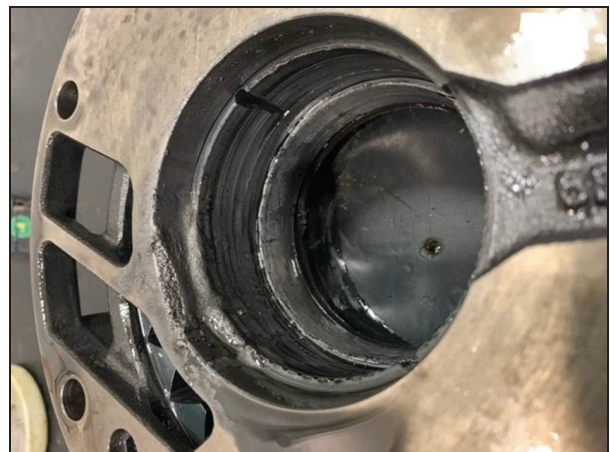
Figure 4: Damage inside the transmission oil pump.
