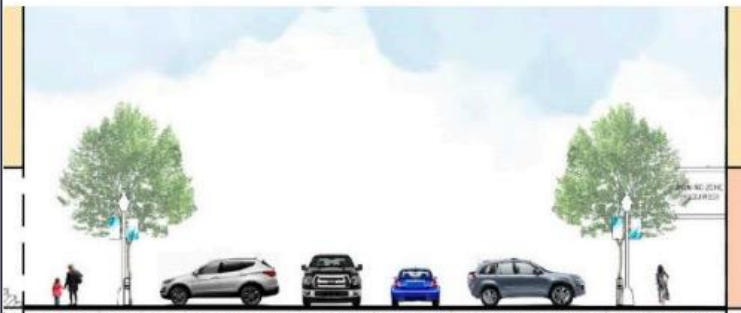
The proposed 27 Avenue 'Centre Street' cross section in the Special Area. The pedestrian environment will feature a minimum 3.0 m wide sidewalk and a 1.7 m wide treed boulevard. Street crossing distances will be reduced by replacing angle parking with curb extensions where necessary.
