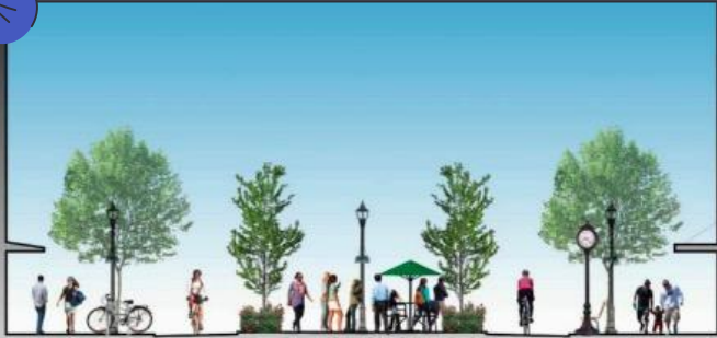
The existing 27 Avenue 'Main Street' cross section in the current DC2 Zone. Pedestrian modal priority is emphasized with 2.5 m wide sidewalks, 2.5 m treed boulevards and 10 m open space median. Vehicles are allowed in the drive lanes beside the median.
