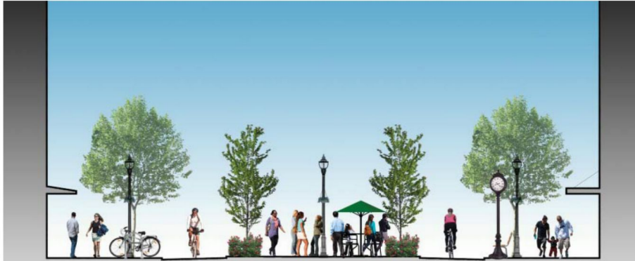
The existing 27 Avenue 'Main Street' cross section in the current DC2 Zone. Pedestrian modal priority is emphasized with 2.5 m wide sidewalks, 2.5 m treed boulevards and 10 m open space median. Vehicles are allowed in the drive lanes beside the median.
