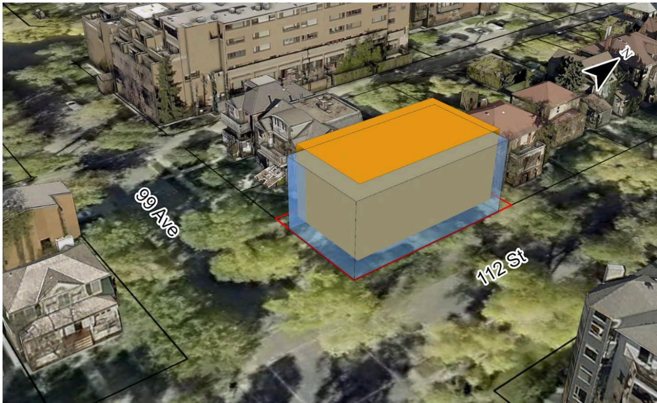
3D model illustrating the impacts of a building (blue box) with no setbacks from 112 Street NW and 99 Avenue NW, as is permitted by the proposed MU h12 f2.2 cf Zone
