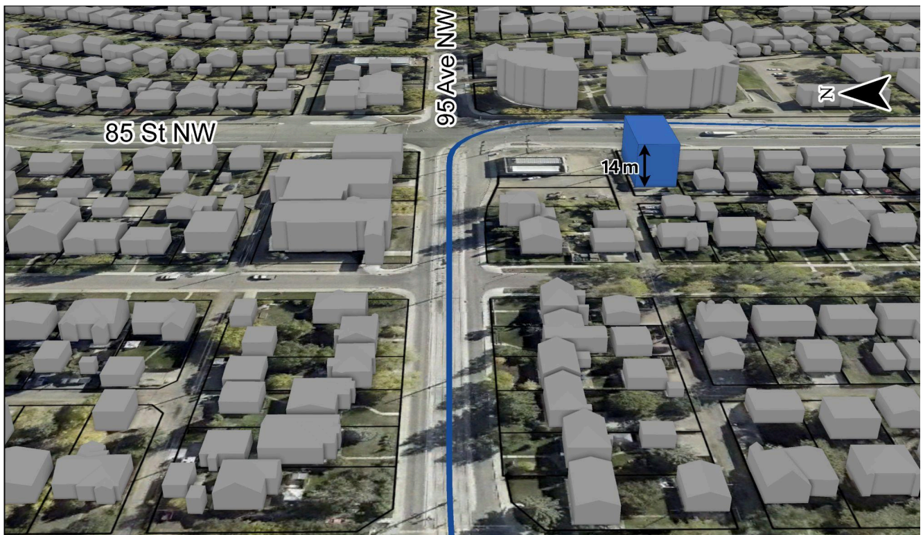
3D Model of proposed RSM h14.0 Zone showing setbacks and maximum height, with increased rear setback to comply with maximum site coverage regulation
