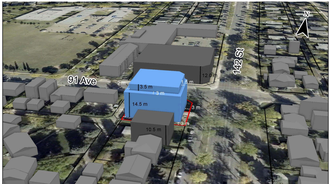
Proposed MU h18 f3.5 cf Zone 3D Model using the maximum front and flanking setbacks (showing the potential built form allowed for the adjacent properties to the north and south)
