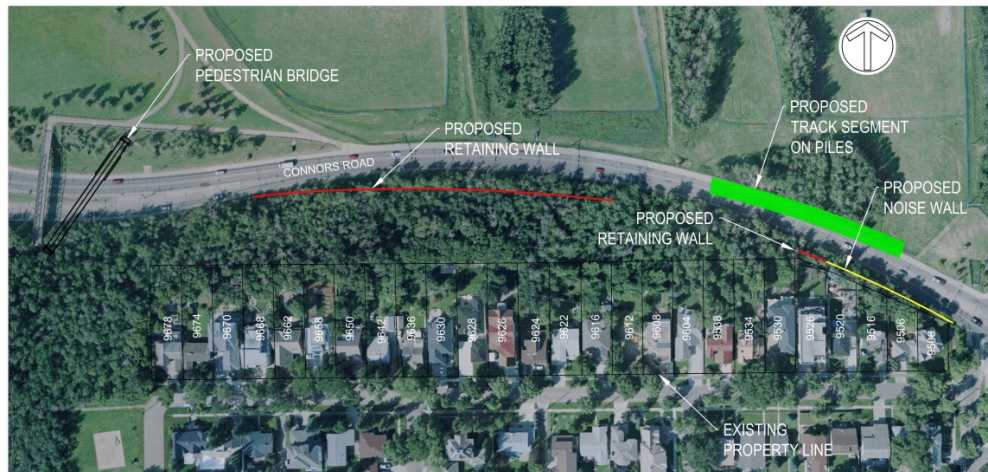
Figure 10. Option 2 - Partial Encroachment to South - Structures
