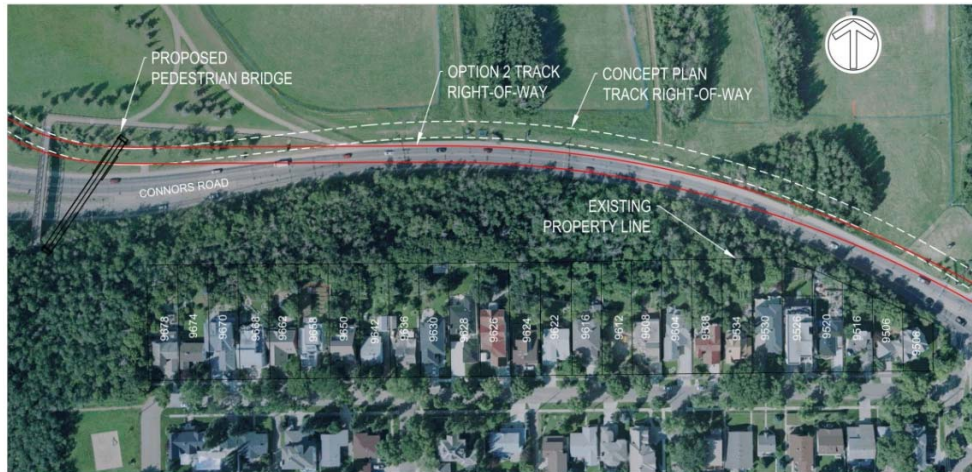
Figure 9. Option 2 - Partial Encroachment to South - Track Alignment
