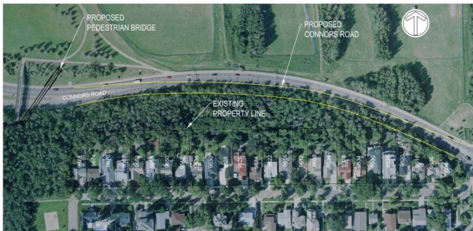
Figure 8. Option 2 - Partial Encroachment to South - Road Alignment
