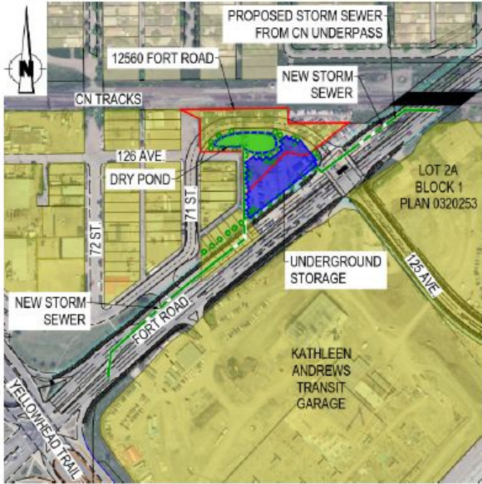
Figure 3: New Stormwater Management System Concept Layout
