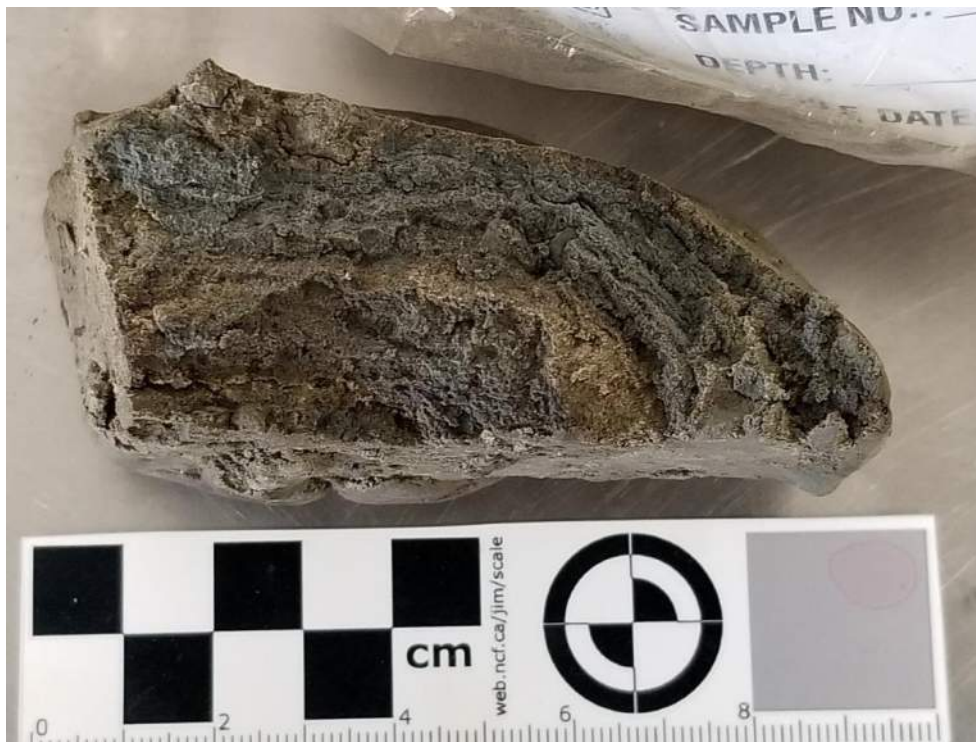
Figure 5: Bedded sandstone of the Horseshoe Canyon Formation. From TH20-03 at 3.0m depth.
