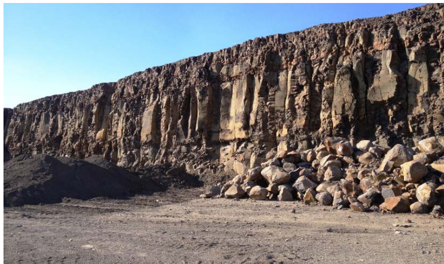
It is also a good practice to work a broad area of the face of a pit or quarry to blend material and reduce variability as it is fed into the processing plant.
