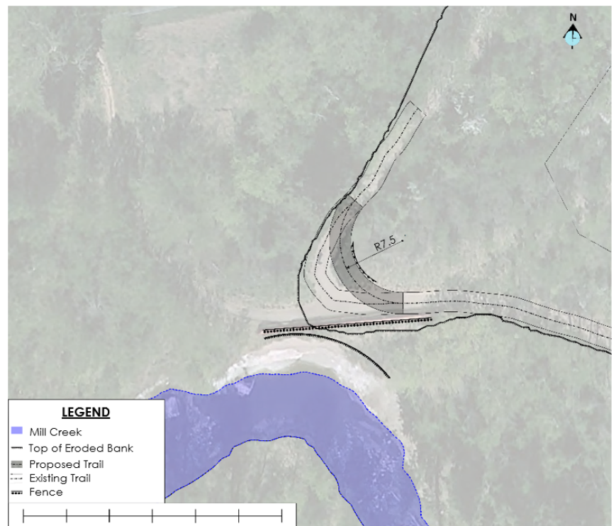
Figure 13 Site 2 - Option 1: Local Trail Realignment – Short Wall
