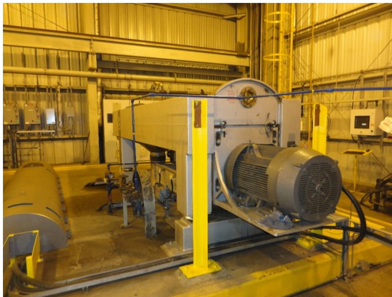
Picture 3-1 (left) View of Centrifuge C with lid removed (bottom left) for annual maintenance.
