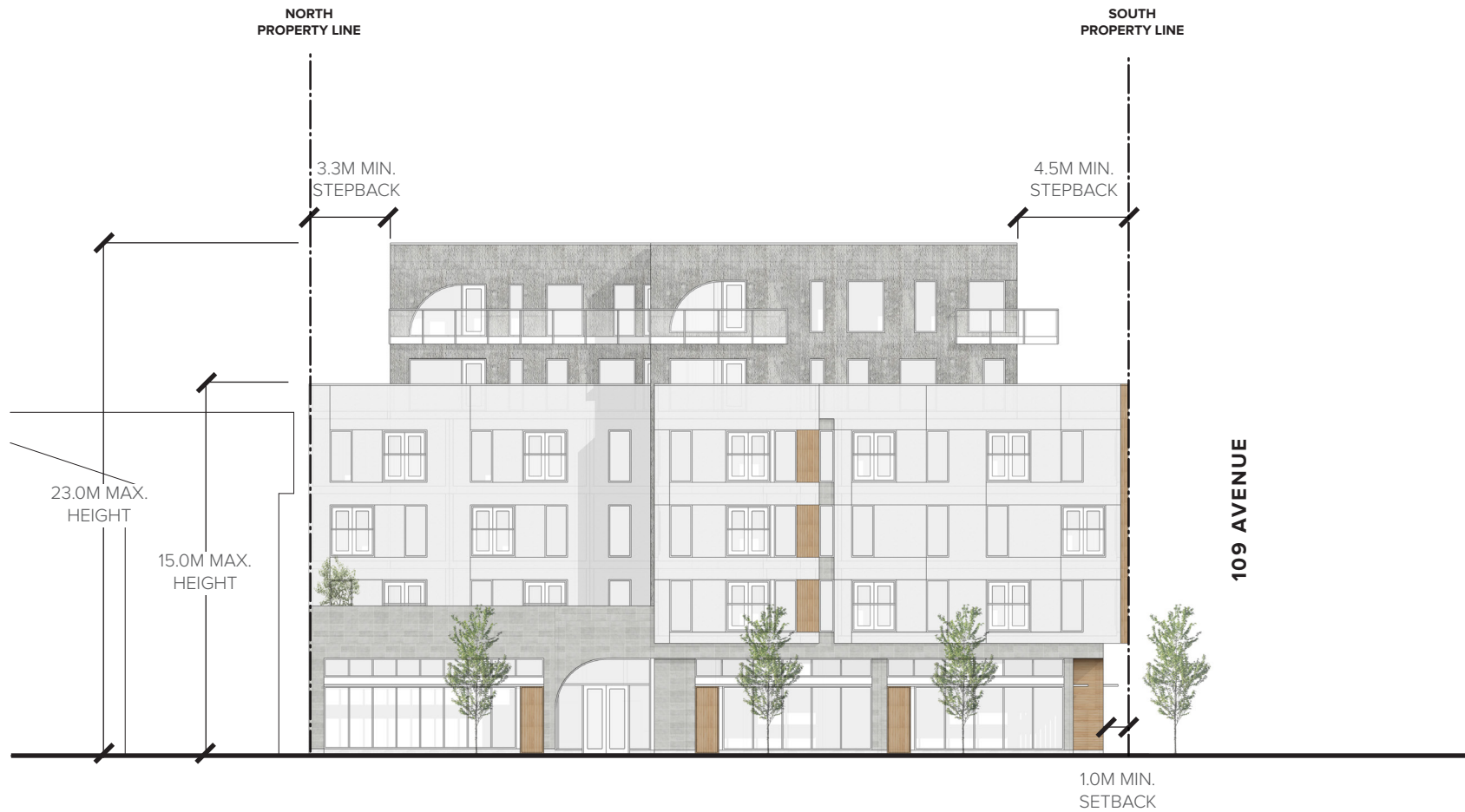
WEST ELEVATION SCALE: NTS
